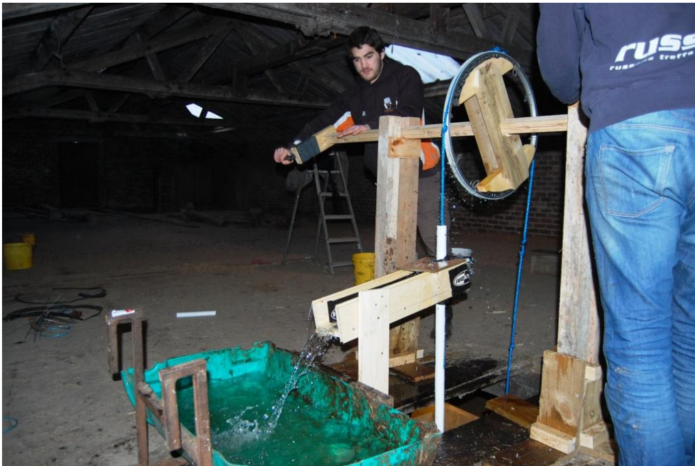
Figure 2.1: Test of the Abakus pump at the Mckeand Farm
