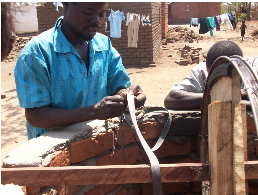
Figure 3.14: Mr. Banda Improving the Grip of the Wheel with Rubber Bands
