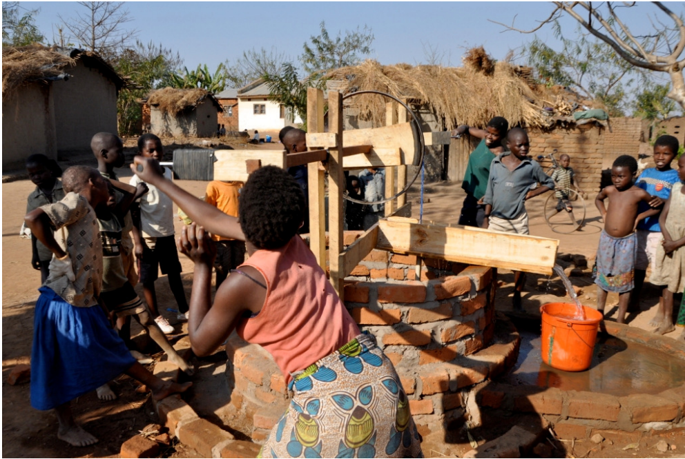
Figure 3.5: The Abakus Pump under Operation
